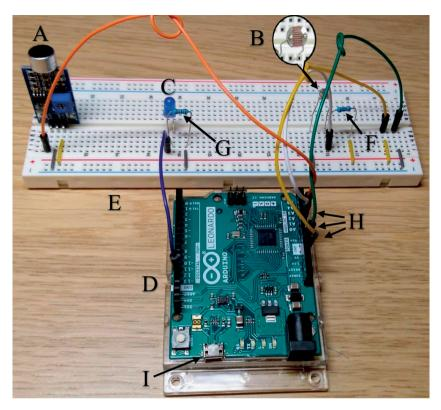
Figure 1 Arduino Microcontroller-Breadboard Circuit. A = Microphone sensor, B = Photoresistor, C = LED, D = Arduino Leonardo, E = Breadboard, F = 10k resistor, G = 220k resistor, H = Jumper wire, I = Micro USB port.
