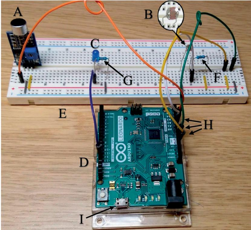
Figure 1 Arduino Microcontroller-Breadboard Circuit. A = Microphone sensor, B = Photoresistor, C = LED, D = Arduino Leonardo, E = Breadboard, F = 10k resistor, G = 220k resistor, H = Jumper wire, I = Micro USB port.
